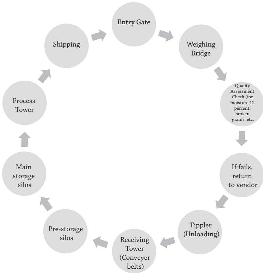
Figure 4.4 Process of Grain Management in Silos
